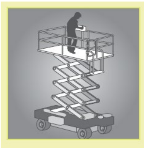
Figure 10: An example of a scissor-lift elevating work platform.
