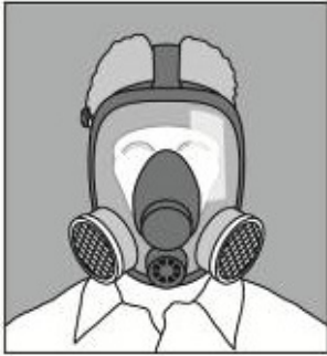
Figure 9 Full-face, powered air-purifying particulate respirator
