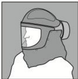
Figure 8 Full-face, particulate filter (cartridge) respirator
