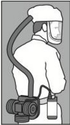
Figure 10 Full-face, positive pressure demand air-line respirator
