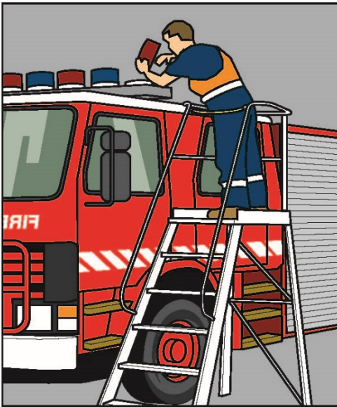
Figure 29: A step platform can provide a stable work surface
