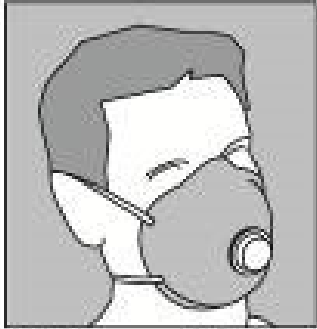
Figure 6 Half-face, particulate filter (cartridge) respirator
