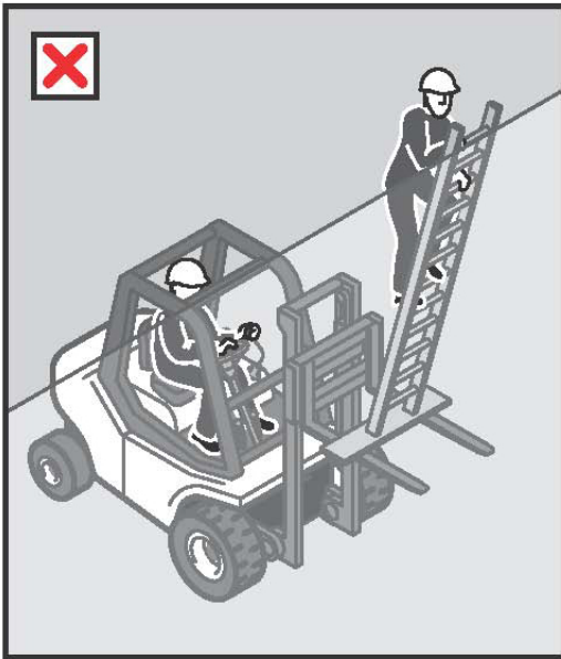
Figure 14: Unacceptable practice with ladder on forklift.
