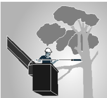
Figure 28 Select tools that are suited to the task, such as long handled saws when pruning trees.
