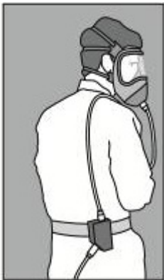
Figure 10 Full-face, positive pressure demand air-line respirator
