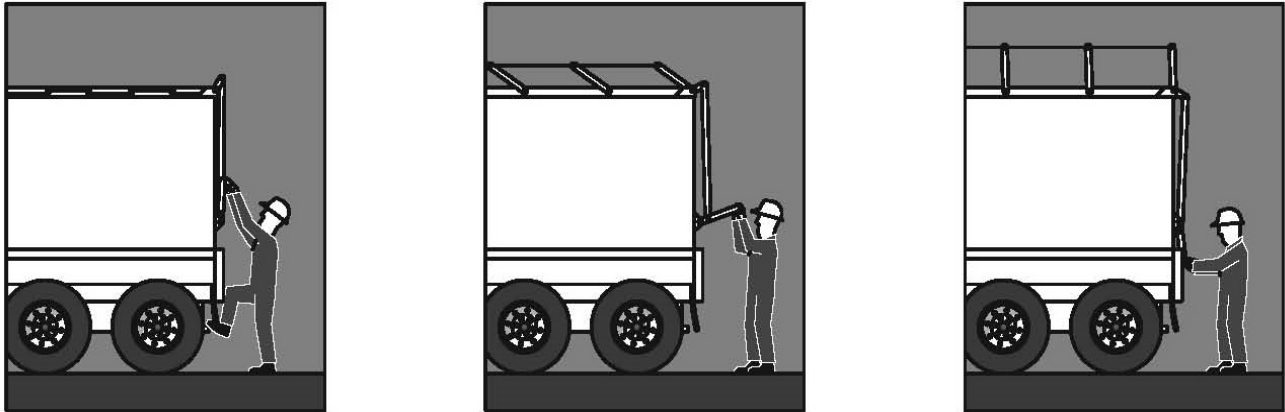
Figure 17: Guard rails installed on top of a tanker to enable safe access to tank hatches.
