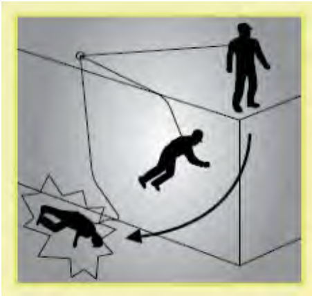
Figure 24: During 'swing back' the length of the lanyard and positioning of the anchor contact may allow the worker to hit the structure.
