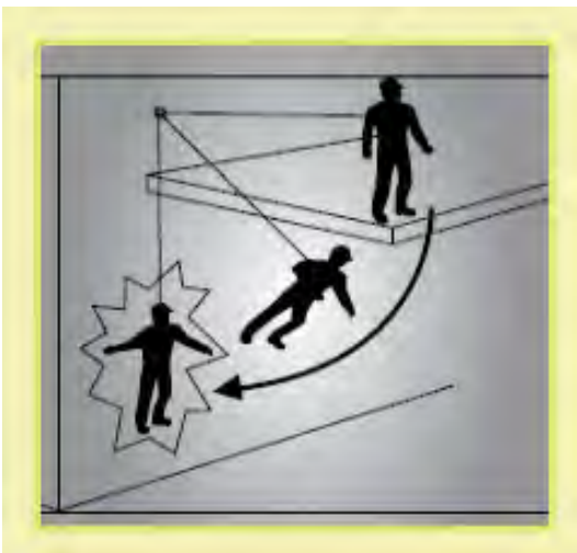
Figure 24: During 'swing back' the length of the lanyard and positioning of the anchor contact may allow the worker to hit the structure.
