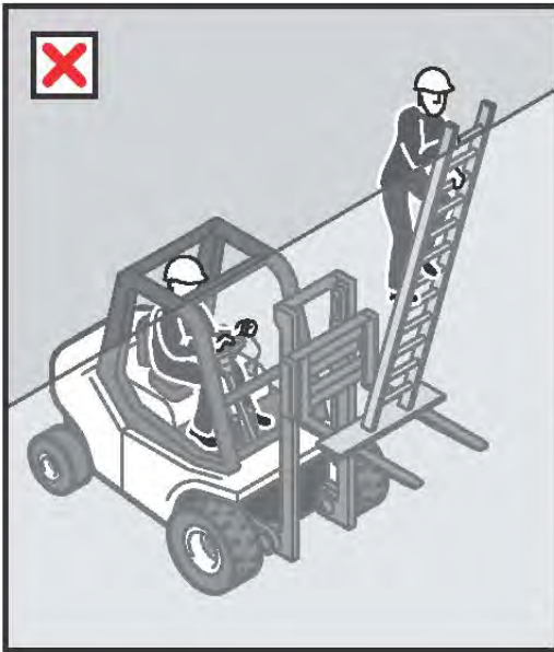
Figure 14: Unacceptable practice with ladder on forklift.
